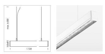
Light band with LED, rated life of the LED L80/B50 > 50000 h, colour rendering index CRI > 80, reflector with homogeneous light distribution pattern, lens optics made of PMMA, luminaire insert sheet steel, powder-coated, white
