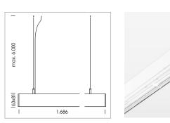
Light band with LED, rated life of the LED L80/B50 > 50000 h, colour rendering index CRI > 80, reflector with homogeneous light distribution pattern, lens optics made of PMMA, luminaire insert sheet steel, powder-coated, white
