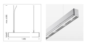
Light band with LED, rated life of the LED L80/B50 > 50000 h, colour rendering index CRI > 80, reflector with double asymmetrical light distribution pattern, lens optics made of PMMA, luminaire insert sheet steel, powder-coated, silver
