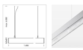
Light band with LED, rated life of the LED L80/B50 > 50000 h, colour rendering index CRI > 80, reflector with homogeneous light distribution pattern, lens optics made of PMMA, luminaire insert sheet steel, powder-coated, silver
