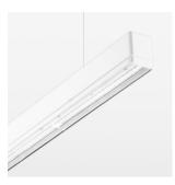
Light band with LED, rated life of the LED L80/B50 > 50000 h, colour rendering index CRI > 80, reflector with homogeneous light distribution pattern, lens optics made of PMMA, luminaire insert sheet steel, powder-coated, white
