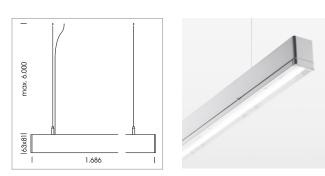
Light band with LED, rated life of the LED L80/B50 > 50000 h, colour rendering index CRI > 80, reflector with homogeneous light distribution pattern, lens optics made of PMMA, luminaire insert sheet steel, powder-coated, silver
