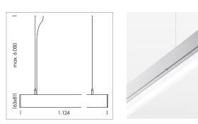
Light band with LED, rated life of the LED L80/B50 > 50000 h, colour rendering index CRI > 80, reflector with homogeneous light distribution pattern, lens optics made of PMMA, luminaire insert sheet steel, powder-coated, silver
