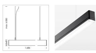
Light band with LED, rated life of the LED L80/B50 > 50000 h, colour rendering index CRI > 80, reflector with homogeneous light distribution pattern, lens optics made of PMMA, luminaire insert sheet steel, powder-coated, black
