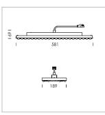
Lay in luminaire with LED, rated life of the LED L80/B50 > 50000 h, colour rendering index CRI > 80, chromaticity tolerance 3 SDCM (initial), wide, homogeneous light distribution pattern, TIR-lens made of PMMA, luminaire housing sheet steel, powder-coated, matt white
