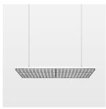
Suspended luminaire with LED, rated life of the LED L80/B50 > 50000 h, colour rendering index CRI > 80, chromaticity tolerance 3 SDCM (initial), double asymmetrical light distribution pattern, lens made of PMMA, luminaire housing sheet steel, powder-coated, matt white, power supply via suspension cables
