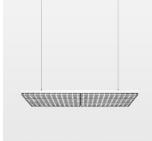
Suspended luminaire with LED, rated life of the LED L80/B50 > 50000 h, colour rendering index CRI > 80, chromaticity tolerance 3 SDCM (initial), double asymmetrical light distribution pattern, lens made of PMMA, luminaire housing sheet steel, powder-coated, matt white, power supply via suspension cables
