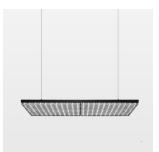
Suspended luminaire with LED, rated life of the LED L80/B50 > 50000 h, colour rendering index CRI > 80, chromaticity tolerance 3 SDCM (initial), extra wide, homogeneous light distribution pattern, TIR-lens made of PMMA, luminaire housing sheet steel, powder-coated, matt black, power supply via suspension cables
