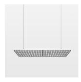
Suspended luminaire with LED, rated life of the LED L80/B50 > 50000 h, colour rendering index CRI > 80, chromaticity tolerance 3 SDCM (initial), extra wide, homogeneous light distribution pattern, TIR-lens made of PMMA, luminaire housing sheet steel, powder-coated, matt white, power supply via suspension cables
