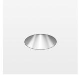
Recessed downlight, flush with ceiling with LED, rated life of the LED L80/B10 > 50000 h, chromaticity tolerance 2 SDCM (initial), reflector with homogeneous light distribution pattern, diffuser lens, translucent, darklight reflector, aluminium, metallised, highgloss, luminaire head die-cast aluminium, black angelized.
