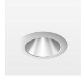
Recessed downlight with LED, rated life of the LED L80/B10 > 50000 h, colour rendering index CRI > 80, chromaticity tolerance 2 SDCM (initial), reflector with homogeneous light distribution pattern, diffuser lens, translucent, darklight reflector, aluminium, metallised, highgloss, luminaire head die-cast aluminium, powder-coated, mounting ring die-cast aluminum, front ring and coverblind plastic, white, separate driver unit
