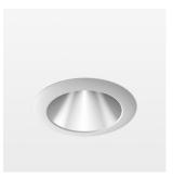
Recessed downlight with LED, rated life of the LED L80/B10 > 50000 h, colour rendering index CRI > 90, chromaticity tolerance 2 SDCM (initial), reflector with homogeneous light distribution pattern, diffuser lens, translucent, darklight reflector, aluminium, metallised, highgloss, luminaire head die-cast aluminium, powder-coated, mounting ring die-cast aluminum, front ring and coverblind plastic, white, separate driver unit
