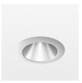
Recessed downlight with LED, rated life of the LED L80/B10 > 50000 h, colour rendering index CRI > 96, chromaticity tolerance 3 SDCM (initial), reflector with homogeneous light distribution pattern, diffuser lens, translucent, darklight reflector, aluminium, metallised, highgloss, luminaire head die-cast aluminium, powder-coated, mounting ring die-cast aluminum, front ring and coverblind plastic, white, separate driver unit
