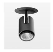
Semi-recessed luminaire with LED, rated life of the LED L80/B10 > 50000 h, chromaticity tolerance 3 SDCM (initial), , reflector with circular light distribution pattern, reflector pure aluminium 99,99% in MIRO-Silver®, segmented and faceted, exchangeable reflector unit in high-sheen black plastic, with glass cover, luminaire head die-cast aluminium, powder-coated, rotation angle 330°, swivel angle +90°/-90°, luminaire housing die-cast aluminium, powder-coated, stratoblack, separate driver unit
