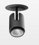
Semi-recessed luminaire with LED, rated life of the LED L80/B10 > 50000 h, chromaticity tolerance 2 SDCM (initial), , reflector with circular light distribution pattern, reflector pure aluminium 99,99% in MIRO-Silver®, segmented and faceted, exchangeable reflector unit in high-sheen black plastic, with glass cover, luminaire head die-cast aluminium, powder-coated, rotation angle 330°, swivel angle +90°/-90°, luminaire housing die-cast aluminium, powder-coated, stratoblack, separate driver unit
