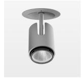
Semi-recessed luminaire with LED, rated life of the LED L80/B10 > 50000 h, chromaticity tolerance 2 SDCM (initial), , reflector with circular light distribution pattern, reflector pure aluminium 99,99% in MIRO-Silver®, segmented and faceted, exchangeable reflector unit in high-sheen black plastic, with glass cover, luminaire head die-cast aluminium, powder-coated, rotation angle 330°, swivel angle +90°/-90°, luminaire housing die-cast aluminium, powder-coated, stratosilver, separate driver unit
