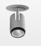
Semi-recessed luminaire with LED, rated life of the LED L80/B10 > 50000 h, chromaticity tolerance 3 SDCM (initial), , reflector with circular light distribution pattern, reflector pure aluminium 99,99% in MIRO-Silver®, segmented and faceted, exchangeable reflector unit in high-sheen black plastic, with glass cover, luminaire head die-cast aluminium, powder-coated, rotation angle 330°, swivel angle +90°/-90°, luminaire housing die-cast aluminium, powder-coated, stratosilver, separate driver unit
