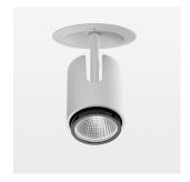
Semi-recessed luminaire with LED, rated life of the LED L80/B10 > 50000 h, chromaticity tolerance 2 SDCM (initial), , reflector with circular light distribution pattern, reflector pure aluminium 99,99% in MIRO-Silver®, segmented and faceted, exchangeable reflector unit in high-sheen black plastic, with glass cover, luminaire head die-cast aluminium, powder-coated, rotation angle 330°, swivel angle +90°/-90°, luminaire housing die-cast aluminium, powder-coated, stratowhite, separate driver unit
