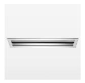
recessed luminaire with LED, rated life of the LED L80/B10 > 50000 h, color rendering index CRI > 80, chromaticity point tolerance 3 SDCM (initial), Reflector with asymerical light distribution pattern, 99.99% pure aluminium reflector made of MIRO-SILVER®, aluminium luminaire housing and frame, anodized, separate driver unit.
