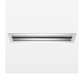
Recessed lumionaire for grid ceiling with LED, rated life of the LED L80/B10 > 50000 h, color rendering index CRI > 80, chromaticity point tolerance 3 SDCM (initial), Reflector with asymerical light distribution pattern, 99.99% pure aluminium reflector made of MIRO-SILVER®, aluminium luminaire housing and frame, anodized, separate driver unit.
