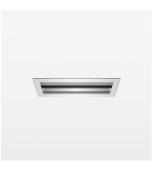
Recessed luminaire with LED, rated life of the LED L80/B10 > 50000 h, colour rendering index CRI > 90, chromaticity tolerance 3 SDCM (initial), reflector with asymmetrical light distribution pattern, reflector pure aluminium 99,99% in MIRO-Silver®, luminaire housing aluminium, aluminium, separate driver unit
