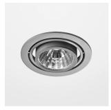
Recessed luminaire with LED, rated life of the LED L80/B10 > 50000h, colour rendering index CRI > 90, chromaticity tolerance 2 SDCM (initial), reflector with circular light distribution pattern, 99,99% pure aluminium, segmented and faceted, cardanic, incl. glass cover, sheet metal powder coated, separate driver unit
