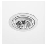
Recessed luminaire with LED, rated life of the LED L80/B10 > 50000h, colour rendering index CRI > 80, chromaticity tolerance 2 SDCM (initial), reflector with circular light distribution pattern, 99,99% pure aluminium, segmented and faceted, cardanic, incl. glass cover, sheet metal powder coated, separate driver unit
