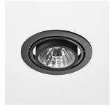
Recessed luminaire with LED, rated life of the LED L80/B10 > 50000h, colour rendering index CRI > 80, chromaticity tolerance 2 SDCM (initial), axially symmetrical reflector with circular light distribution pattern, 99,99% pure aluminium, segmented and faceted, cardanic, incl. glass cover, sheet metal powder coated, separate driver unit
