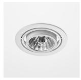
Recessed luminaire with LED, rated life of the LED L80/B10 > 50000h, colour rendering index CRI > 90, chromaticity tolerance 2 SDCM (initial), axially symmetrical reflector with circular light distribution pattern, 99,99% pure aluminium, segmented and faceted, cardanic, incl. glass cover, sheet metal powder coated, separate driver unit
