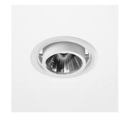
Recessed luminaire with LED, rated life of the LED L80/B10 > 50000h, colour rendering index CRI > 90, chromaticity tolerance 2 SDCM (initial), reflector with circular light distribution pattern, 99,99% pure aluminium, segmented and faceted, infinitely adjustable sheet steel luminaire housing, incl. glass cover, sheet metal powder coated, separate driver unit
