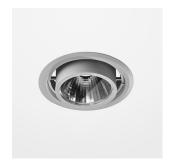
Recessed luminaire with LED, rated life of the LED L80/B10 > 50000h, colour rendering index CRI > 80, chromaticity tolerance 2 SDCM (initial), axially symmetrical reflector with circular light distribution pattern, 99,99% pure aluminium, segmented and faceted, infinitely adjustable sheet steel luminaire housing, incl. glass cover, sheet metal powder coated, separate driver unit
