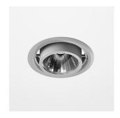
Recessed luminaire with LED, rated life of the LED L80/B10 > 50000h, colour rendering index CRI > 90, chromaticity tolerance 2 SDCM (initial), axially symmetrical reflector with circular light distribution pattern, 99,99% pure aluminium, segmented and faceted, infinitely adjustable sheet steel luminaire housing, incl. glass cover, sheet metal powder coated, separate driver unit
