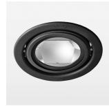
Recessed luminaire with LED, rated life of the LED L80/B10 > 50000 h, colour rendering index CRI > 80, chromaticity tolerance 2 SDCM (initial), reflector with circular light distribution pattern, reflector pure aluminium 99,99% in MIRO-Silver®, swivel angle +25°/-25°, luminaire housing sheet steel, powder-coated, stratoblack, separate driver unit
