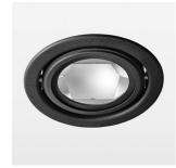
Recessed luminaire with LED, rated life of the LED L80/B10 > 50000 h, colour rendering index CRI > 90, chromaticity tolerance 2 SDCM (initial), reflector with circular light distribution pattern, reflector pure aluminium 99,99% in MIRO-Silver®, swivel angle +25°/-25°, luminaire housing sheet steel, powder-coated, stratoblack, separate driver unit
