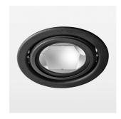
Recessed luminaire with LED, rated life of the LED L80/B10 > 50000 h, chromaticity tolerance 2 SDCM (initial), reflector with circular light distribution pattern, reflector pure aluminium 99,99% in MIRO-Silver®, swivel angle +25°/-25°, luminaire housing sheet steel, powder-coated, stratoblack, separate driver unit
