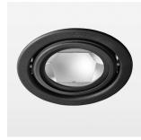
Recessed luminaire with LED, rated life of the LED L80/B10 > 50000 h, chromaticity tolerance 3 SDCM (initial), reflector with circular light distribution pattern, reflector pure aluminium 99,99% in MIRO-Silver®, swivel angle +25°/-25°, luminaire housing sheet steel, powder-coated, stratoblack, separate driver unit
