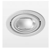
Recessed luminaire with LED, rated life of the LED L80/B10 > 50000 h, chromaticity tolerance 2 SDCM (initial), reflector with circular light distribution pattern, reflector pure aluminium 99,99% in MIRO-Silver®, swivel angle +25°/-25°, luminaire housing sheet steel, powder-coated, stratowhite, separate driver unit
