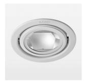
Recessed luminaire with LED, rated life of the LED L80/B10 > 50000 h, chromaticity tolerance 2 SDCM (initial), reflector with circular light distribution pattern, reflector pure aluminium 99,99% in MIRO-Silver®, swivel angle +25°/-25°, luminaire housing sheet steel, powder-coated, stratowhite, separate driver unit
