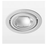
Recessed luminaire with LED, rated life of the LED L80/B10 > 50000 h, chromaticity tolerance 3 SDCM (initial), reflector with circular light distribution pattern, reflector pure aluminium 99,99% in MIRO-Silver®, swivel angle +25°/-25°, luminaire housing sheet steel, powder-coated, stratowhite, separate driver unit
