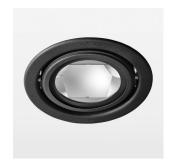
Recessed luminaire with LED, rated life of the LED L70/B10 > 50000 h, chromaticity tolerance 3 SDCM (initial), reflector with circular light distribution pattern, reflector pure aluminium 99,99% in MIRO-Silver®, luminaire head die-cast aluminium, powder-coated, swivel angle +25°/-25°, luminaire housing sheet steel, powder-coated, stratoblack, separate driver unit
