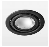
Recessed luminaire with LED, rated life of the LED L80/B10 > 50000 h, colour rendering index CRI > 80, chromaticity tolerance 2 SDCM (initial), reflector with circular light distribution pattern, reflector pure aluminium 99,99% in MIRO-Silver®, swivel angle +25°/-25°, luminaire housing sheet steel, powdercoated, stratoblack, separate driver unit
