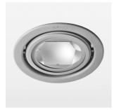
Recessed luminaire with LED, rated life of the LED L80/B10 > 50000 h, colour rendering index CRI > 80, chromaticity tolerance 2 SDCM (initial), reflector with circular light distribution pattern, reflector pure aluminium 99,99% in MIRO-Silver®, swivel angle +25°/-25°, luminaire housing sheet steel, powdercoated, stratosilver, separate driver unit
