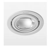
Recessed luminaire with LED, rated life of the LED L80/B10 > 50000 h, colour rendering index CRI > 90, chromaticity tolerance 2 SDCM (initial), reflector with circular light distribution pattern, reflector pure aluminium 99,99% in MIRO-Silver®, swivel angle +25°/-25°, luminaire housing sheet steel, powder-coated, stratowhite, separate driver unit
