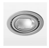
Recessed luminaire with LED, rated life of the LED L80/B10 > 50000 h, colour rendering index CRI > 80, chromaticity tolerance 2 SDCM (initial), reflector with oval light distribution pattern, reflector pure aluminium 99,99% in MIRO-Silver®, swivel angle +25°/-25°, luminaire housing sheet steel, powder-coated, stratosilver, separate driver unit
