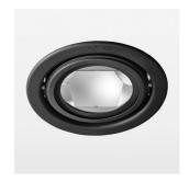
Recessed luminaire with LED, rated life of the LED L80/B10 > 50000 h, colour rendering index CRI > 90, chromaticity tolerance 2 SDCM (initial), reflector with oval light distribution pattern, reflector pure aluminium 99,99% in MIRO-Silver®, swivel angle +25°/-25°, luminaire housing sheet steel, powder-coated, stratoblack, separate driver unit
