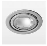
Recessed luminaire with LED, rated life of the LED L80/B10 > 50000 h, colour rendering index CRI > 90, chromaticity tolerance 2 SDCM (initial), reflector with circular light distribution pattern, reflector pure aluminium 99,99% in MIRO-Silver®, swivel angle +25°/-25°, luminaire housing sheet steel, powdercoated, stratosilver, separate driver unit
