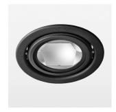
Recessed luminaire with LED, rated life of the LED L80/B10 > 50000 h, chromaticity tolerance 2 SDCM (initial), reflector with circular light distribution pattern, reflector pure aluminium 99,99% in MIRO-Silver®, swivel angle +25°/-25°, luminaire housing sheet steel, powder-coated, stratoblack, separate driver unit
