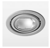
Recessed luminaire with LED, rated life of the LED L80/B10 > 50000 h, colour rendering index CRI > 90, chromaticity tolerance 2 SDCM (initial), reflector with circular light distribution pattern, reflector pure aluminium 99,99% in MIRO-Silver®, swivel angle  $+25^{\circ}/-25^{\circ}$ , luminaire housing sheet steel, powder-coated, stratosilver, separate driver unit
