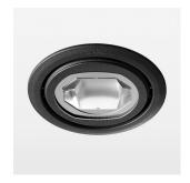
Recessed luminaire with LED, rated life of the LED L80/B10 > 50000 h, chromaticity tolerance 2 SDCM (initial), reflector with oval light distribution pattern, reflector pure aluminium 99,99% in MIRO-Silver®, rotation angle 170°, swivel angle +30°/-30°, luminaire housing sheet steel, powder-coated, stratoblack, separate driver unit
