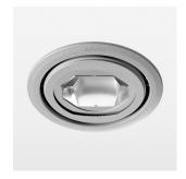
Recessed luminaire with LED, rated life of the LED L80/B10 > 50000 h, chromaticity tolerance 2 SDCM (initial), reflector with circular light distribution pattern, reflector pure aluminium 99,99% in MIRO-Silver®, rotation angle 170°, swivel angle +30°/-30°, luminaire housing sheet steel, powder-coated, stratosilver, separate driver unit
